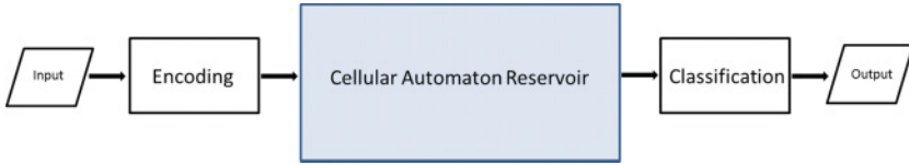
Figure 2: General framework for cellular automata-based reservoir computing.
