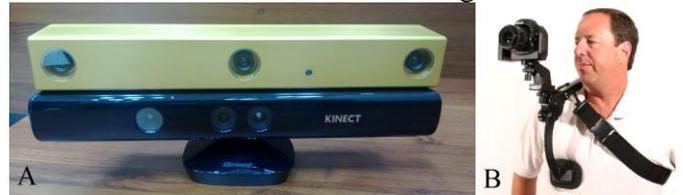
Fig. 1 A. Kinect plus Bumblebee XB3 stereo rig used in the system. B. Padded shoulder image stabilizer for image acquisition. Brand name RPS [26]
